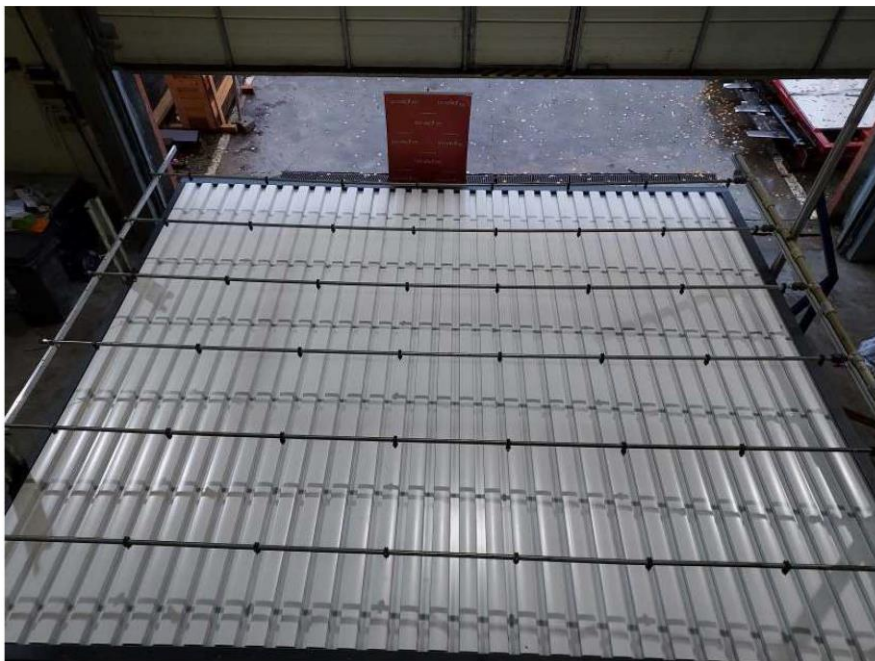
Photo 2. Top view of the sample with the water spray system.
