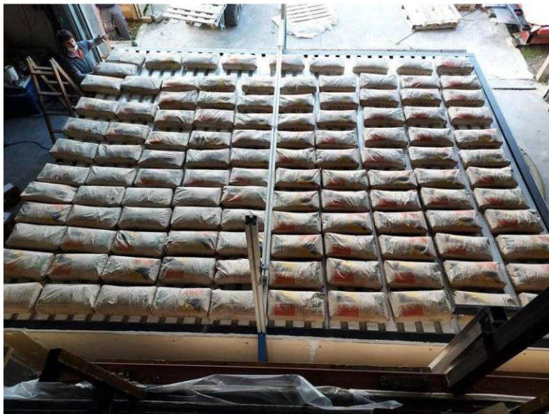
Photo 8. Photograph taken during the snow load resistance test.
