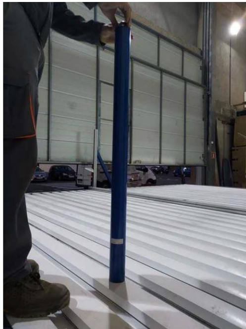
Photo 10. Photograph taken during the hard body strength test.
