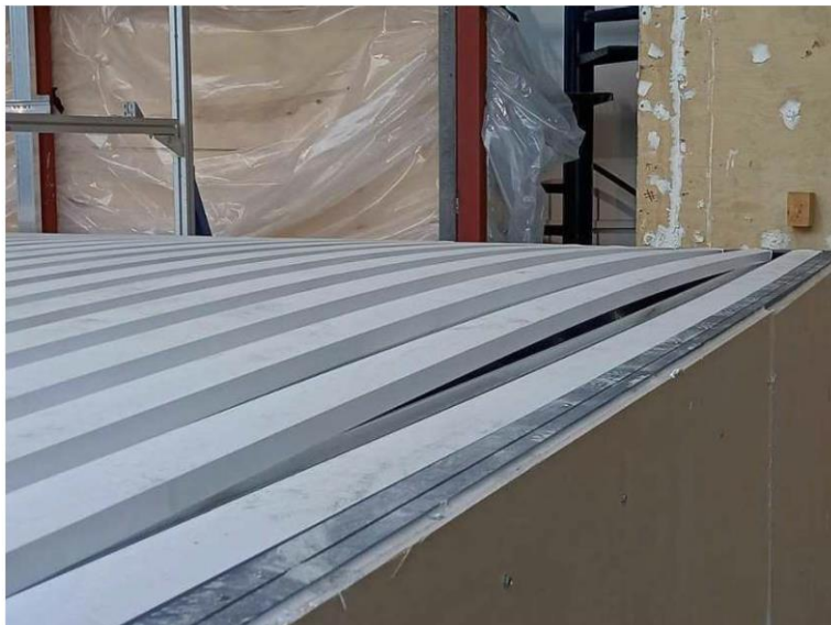
Photo 6. Sample failure before reaching 2600 Pa of suction.
