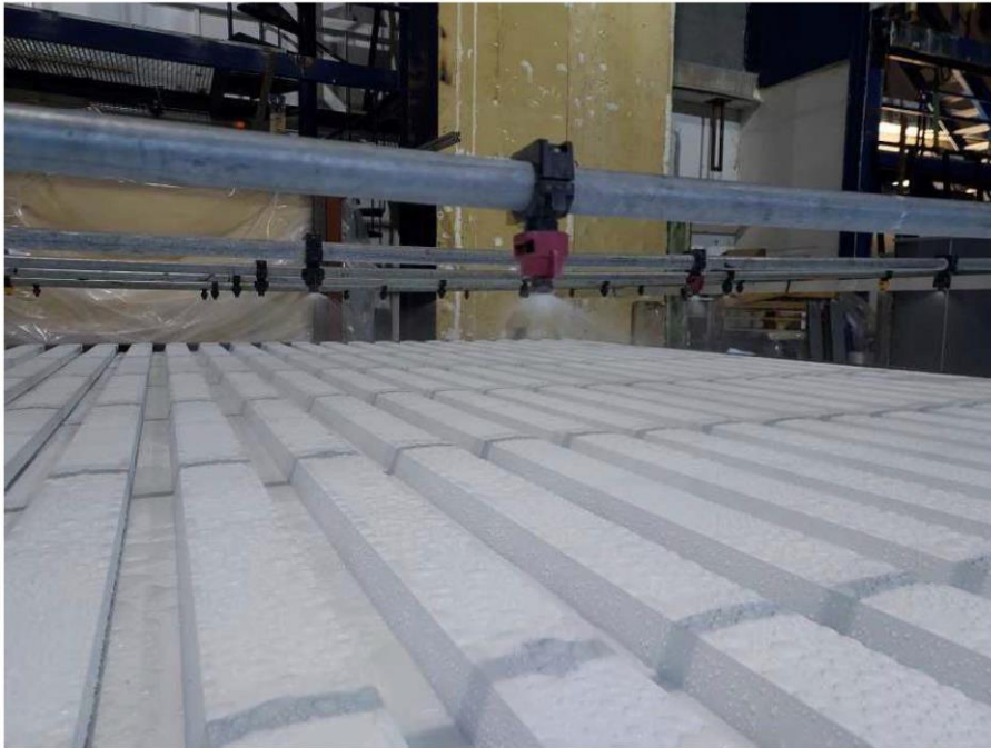
Photo 3. Photograph taken during the watertightness test.
