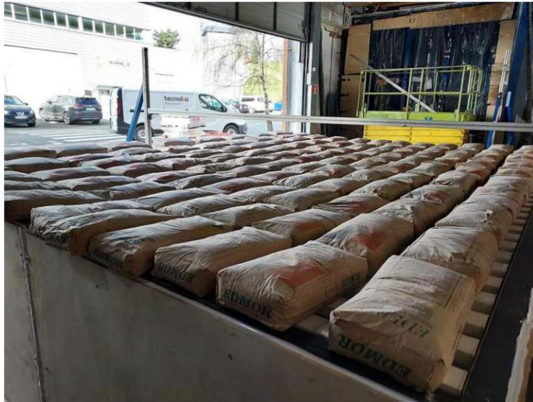
Photo 7. Photograph taken during the snow load resistance test.
